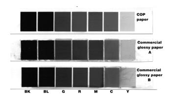
Figure 9. Water-Fastness Test; The test samples were immersed in water for 1 min.
