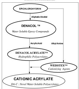
The principal synthetic root of cationic acrylate, DA-C, is shown in above diagram. The schematic formula of DA-C is as follows.
