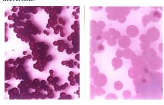
Figure 5. Swelling of spherical COP by aqueous ink; left: before swelling; right: after absorbing magenta ink
